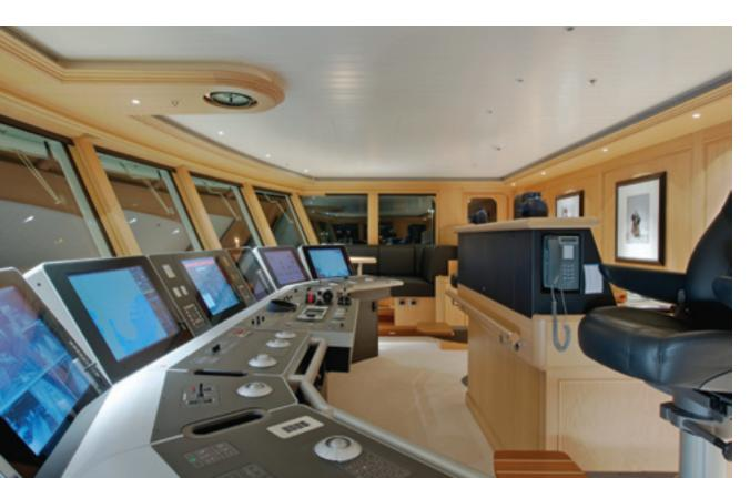
**LEFT:** The bridge with its state-of-the-art navigation equipment has inward sloping windows commonly found on true exploration vessels.
